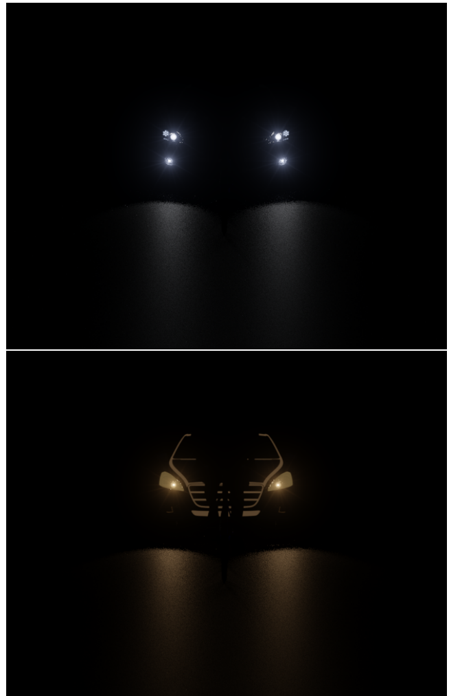
Figure 1: Illustration of a visual masking scenario in traffic. Identical scenes of a car and a bicyclist rendered with different lamp layouts. Note that the silhouette of the cyclist is visible in the bottom image while it is practically invisible in the top image. (Car object is as used in the experiment, albeit with more realistic rendering for illustration purposes.)
